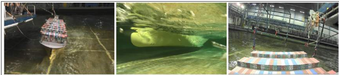
Figure 44: Scale model in MARIN test basin with video above water, underwater and from the bridge (Source: MARIN)
