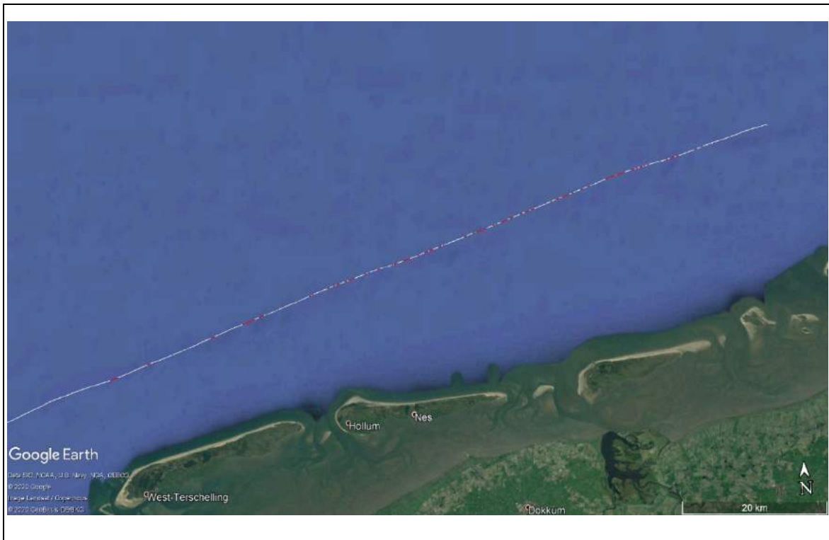
Figure 43: Periods where the rolling motion was intense enough to be detectable by the human ear through shifting objects on the bridge are indicated in red. (Source: Google Earth)
