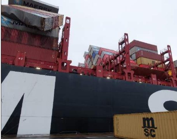
Figure 9: Collapsed rows in bay 42 and 50. (Source: BSU)
