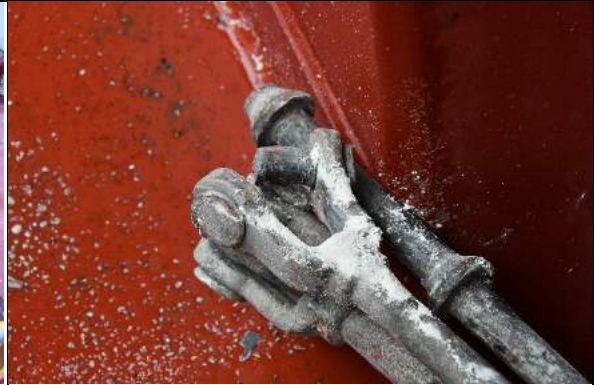
Figure 14: Broken mount from lashing bridge (Source: German Waterway Police)
