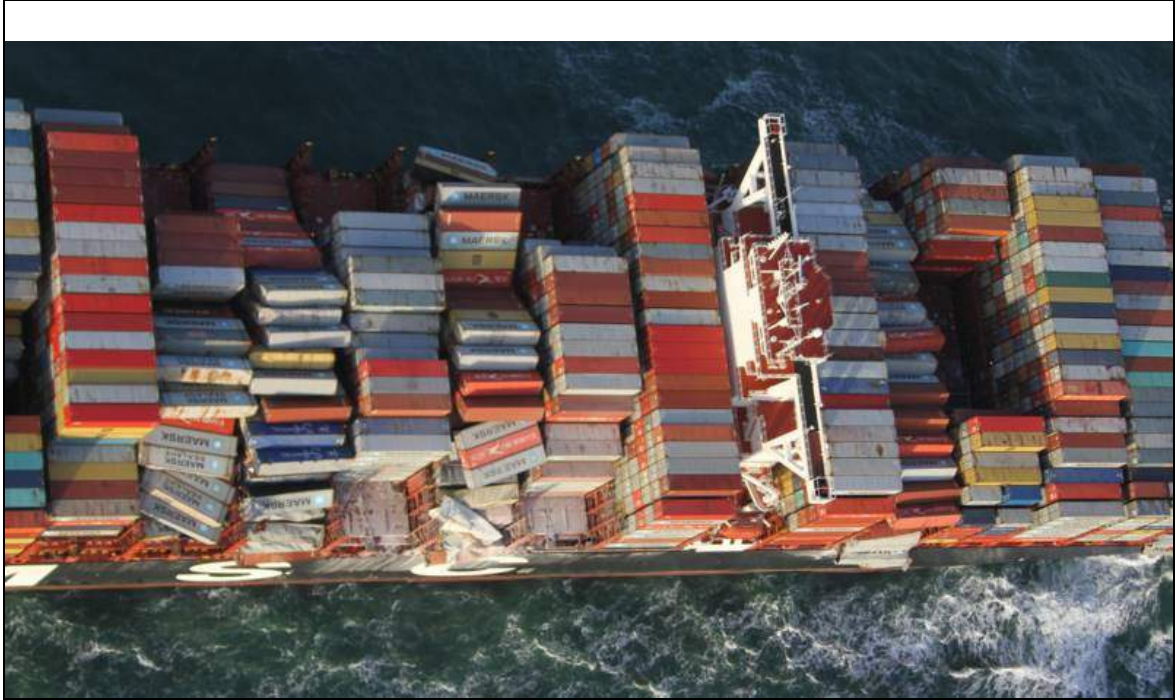
Figure 3: Top view MSC ZOE following the loss overboard of the containers. (Source: Netherlands Coastguard)
