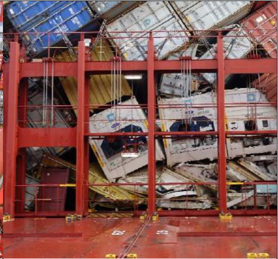
Figure 8: Collapsed containers in bay 26. (Source: BSU)
