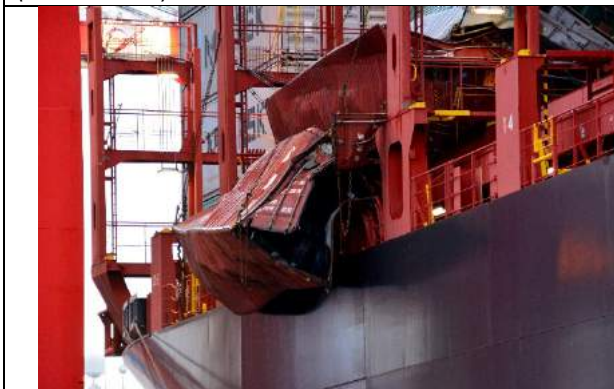
Figure 9: Collapsed rows in bay 42 and 50. (Source: BSU)
